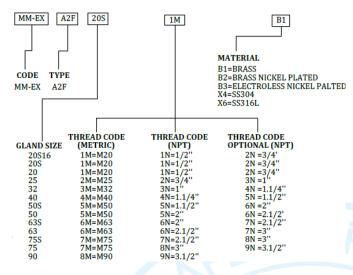
2. Model Nomenclature of MM-EX E1FUNV \*\*\* \*\* series cable glands for armoured cable:
